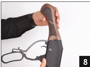
8 - Same way as explained previously to take off the grip remove the nut /screw from inside of grip.
