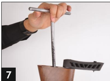
7 - First remove the screw of rubber pad and then take out the screw of stock/butt.
