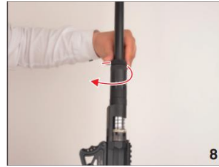
8. Unscrew the gas system retaining nut by turning in arrow direction
