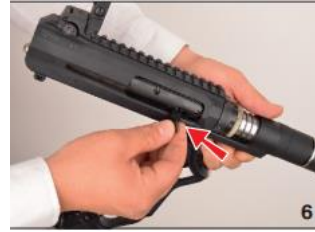
6. Remove the charging handle by pulling it
