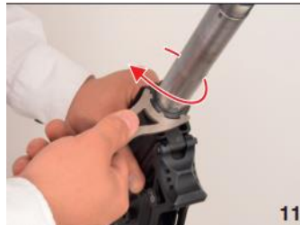
11. Remove the barrel nut with the help of wrench
