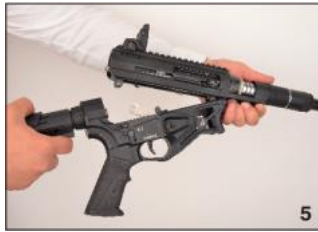
5. Separate Upper and Lower Receiver
