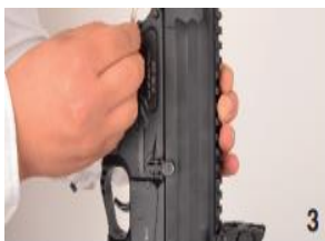
3. Loosen the handguard screw
