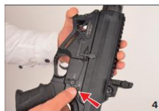
4. Pull the upper receiver pivot pins
