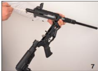
7. Takeout bolt and action bar
