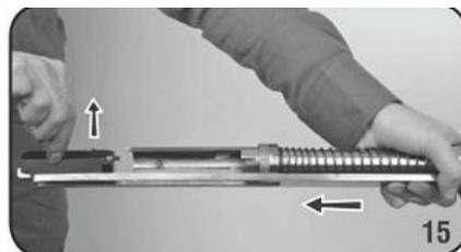
15) Separate the barrel from upper receiver
