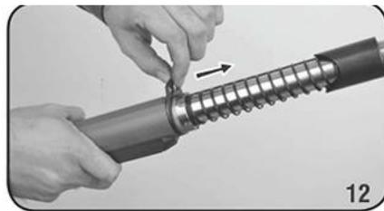
12) Remove the nut in the direction arrow
