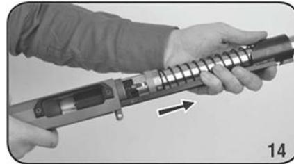
14) Take out action bar by pushing in the direction of arrow
