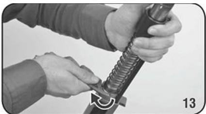
13) Take out the Barrel Assembly Nut by Turning in the clockwise
