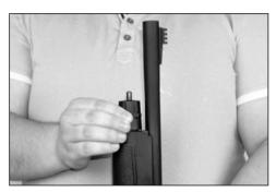
3) Open the action slightly then push the barrel forward and of the receiver.
