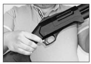
3) Pull the forend/charging handle backwards and check the chamber and magazine tube is unloaded.
