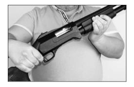
**4)** While folding or unfolding your weapon do not put any item or part of anything between upper and lower receiver. Pull the receiver lock back for unfolding.
