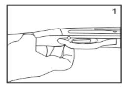
C- When you are ready to fire the gun, press the safety button to the "off position so that the safety protrudes from the left side of the gun and the RED BAND MARKING IS SHOWING.
