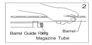
Slide the barrel guide ring over the magazine tube. Clean the barrel following the instructions on Page 8.
